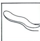
BC-21-328 1 mm wide x 5 mm long, strongly curved tip, offset to the right
