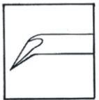
BC-21-380 0.25 mm long point Angled 30 degrees Malleable shaft
