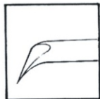
BC-21-382 0.66 mm long point Angled 30 degrees Malleable shaft
