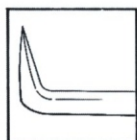
BC-21-395 1 mm long point Angled 90 degrees Malleable shaft
