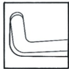
BC-21-391 Small 0.5 mm wide x 1.5 mm long, flattened tip Angled 90 degrees
