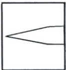
BC-21-392 Straight point 85 mm from angle to tip
