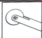
BC-21-334 3 mm diameter roller blade in line with handle Curved shaft
