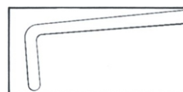
BC-21-487 1 mm long point Angled right 90 degrees Malleable shaft, angled 8 degrees 53 mm from angle to tip Overall length 168 mm, 6.6 inches
