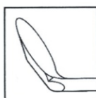
BC-21-327 5 mm diameter blade Angled up 45 degrees
